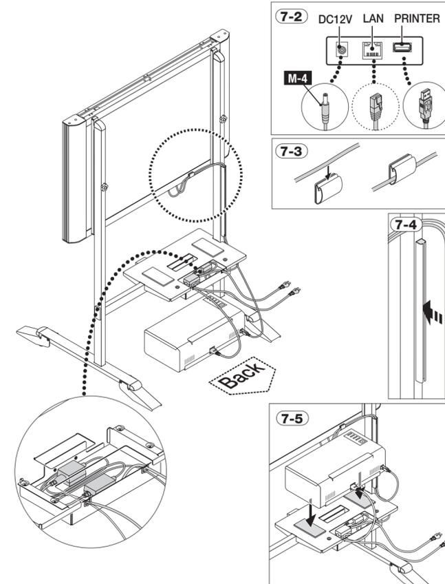
When attaching the adapter holder on the copyboard
