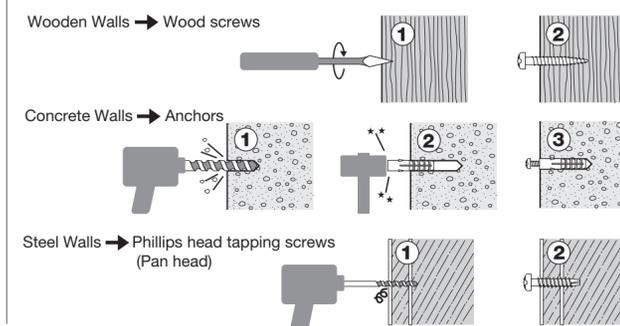
Please install the main unit to posts or studs when the wall surface is of insufficient strength.
