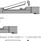
4. Adjust to the polarity indication of the holder (+, -) and insert the battery correctly.
