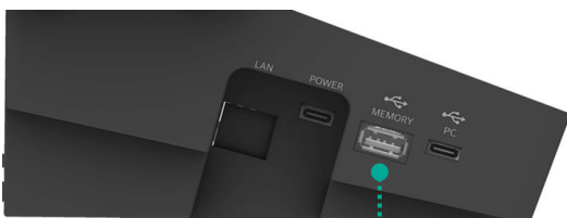
USB Flash Drive Port (Type A)
